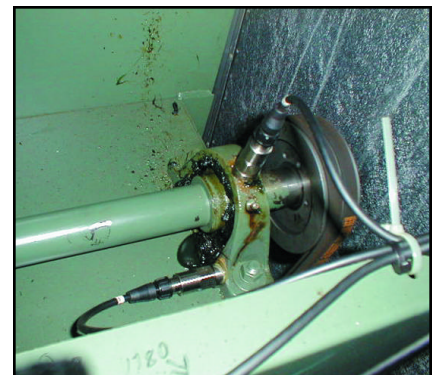
Figure 3 - To provide the optimum vibration transfer between the machine surface and the accelerometer, a mounting system that utilizes the full frequency span of the accelerometer needed to be considered.
